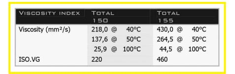
The vibration case lubricant installed at the factory is Total Carter SH 220 for systems with forced lubrication and Total Carter SH 460 for systems with splash lubrication. When replacing the lubricant, a gear oil with the following specifications must be used:
